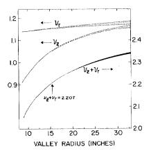
Fig. 1. Radial dependence of  $v_z$  and  $v_r$  for protons in the injector cyclotron (left ordinate). Shaded regions indicate the spread in values for proton energies between 3 and 15 MeV. The corresponding spread in values for  $(v_z + v_r)$ , which determines the proton resonance position, is also shown (right ordinate).
