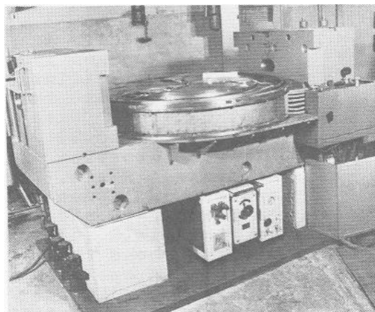
Fig.1. General view of the cyclotron electromagnet during assembly. The sectors and harmonic coils of the lower pole are shown.
