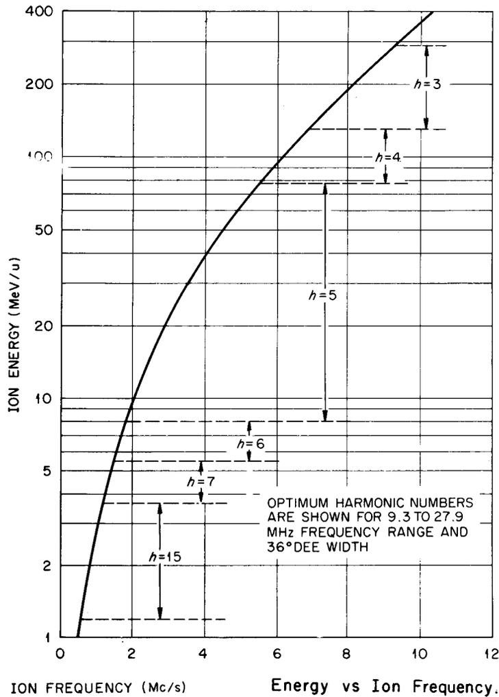
Fig. 3. Ion energy and optimum acceleration harmonics,  $h$ , as a function of orbit frequency
