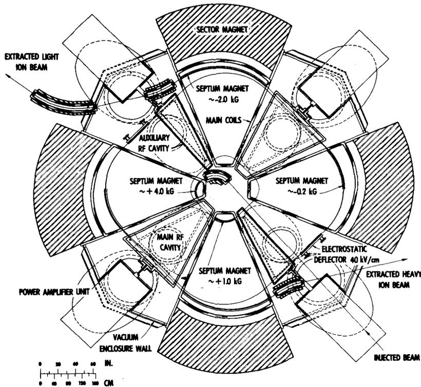
Fig. 1. Plan of the heavy ion cyclotron
