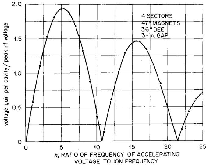
Fig. 5. Ratio of voltage gain per rf cavity to peak rf voltage as a function of harmonic number, or ratio of radio frequency to orbit frequency
