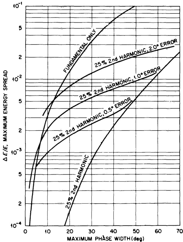
Fig. 6. The energy deviation as a function of the phase width for 25% second harmonic amplitude and for several values of phase error
