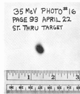
Fig. 8. 35 MeV beam photograph taken at the straight-through target area.
