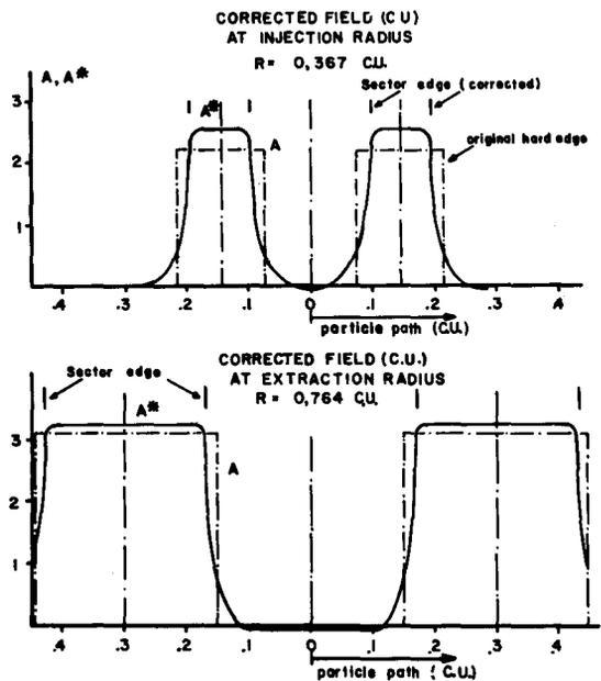
Fig. 6 Field configuration along a particle path at the injection radius and at the extraction radius.
