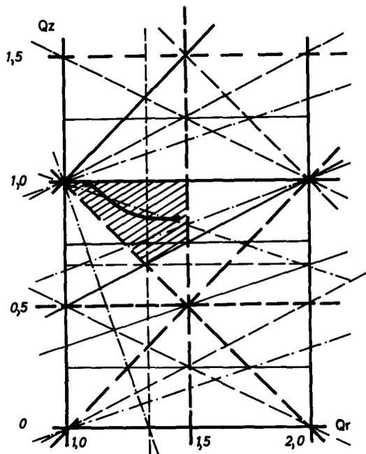
Fig. 3  $Q_z, Q_r$  diagram for an 8-fold sector geometry showing also higher order coupling resonances. Proposed working area with computed working path for the sector geometry under consideration.
