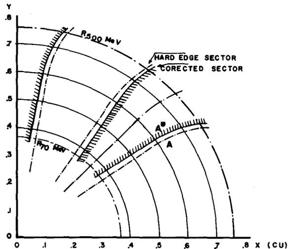
Fig. 4 Hard edge sector geometry and sector shape after correction taking account of the fringe field of the magnets.
