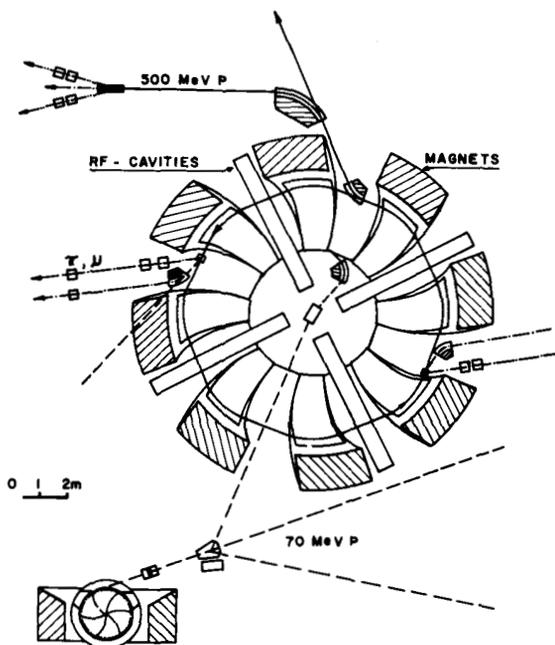
Fig. 8 Schematic layout of the isochronous ring accelerator with injector.
