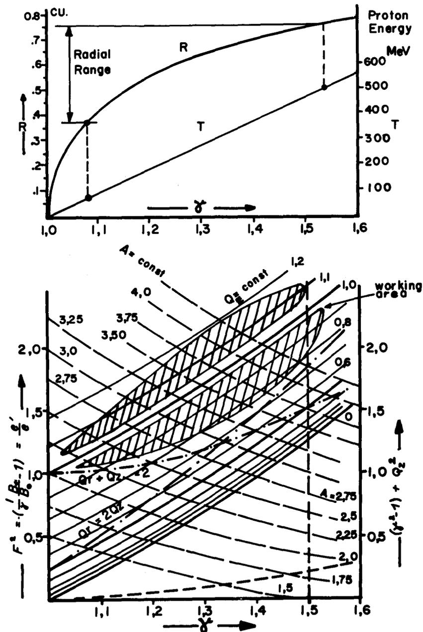
Fig. 2 Working graph for the layout of an 8-sector hard-edge isochronous field. Equivalent radius, flutter factor and spiral-angle defining function  $(\gamma^2 - 1) + Q_z^2$  vs.  $\gamma = \frac{v}{v_0} + 1$ .
