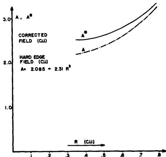
Fig. 5 Radial increase of the field in a magnet section, curve A shows the hard edge case, and  $A^*$  the case corrected for the fringe field of the magnets.
