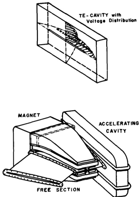
Fig. 9 Schematic sketch of the main components of the isochronous ring accelerator.
