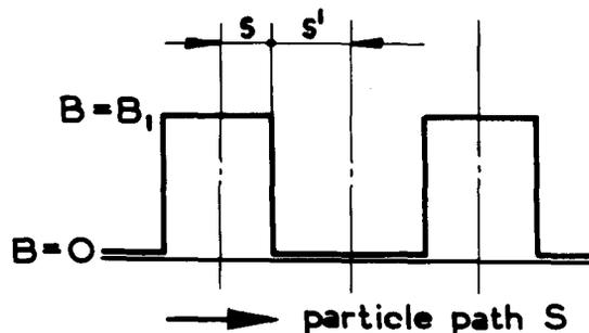
Fig. 1 Hard edge flutter function.
