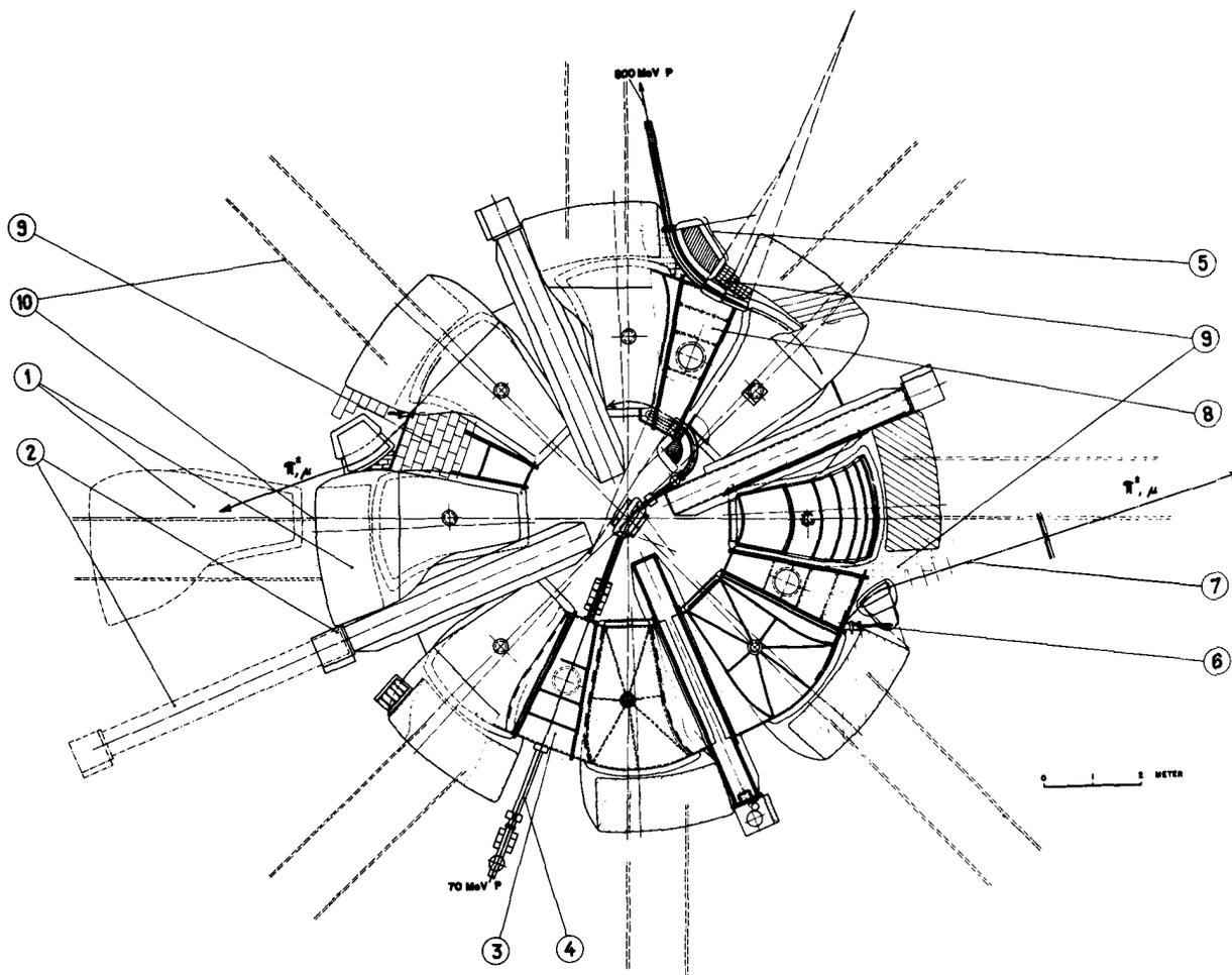
Fig 10 Isochronous ring accelerator. Plan view with sections.
