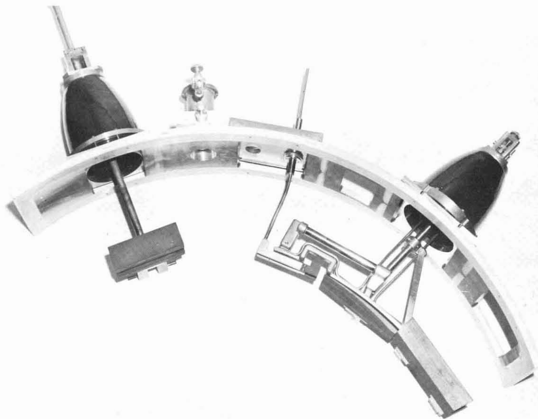
Fig. 3 Photograph of dee-box cover, with the peeler, deflector and septum in position.
