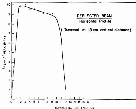
Fig. 264. Horizontal profile of deflected deuteron beam, shown in previous figure.
