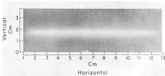
Fig. 262. Cross section of deflected beam, at target box.
