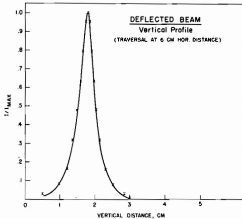
Fig. 263. Vertical profile of deflected deuteron beam, shown in previous figure.
