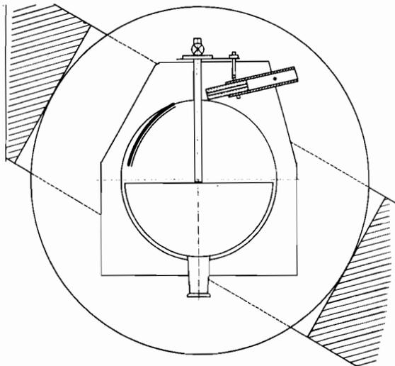
Fig. 212. Beam extraction system of the University of Rochester Variable-Energy Cyclotron.
