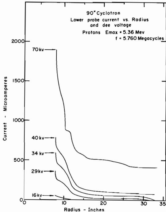
Fig. 202. Beam current vs radius as a function of dee voltage.
