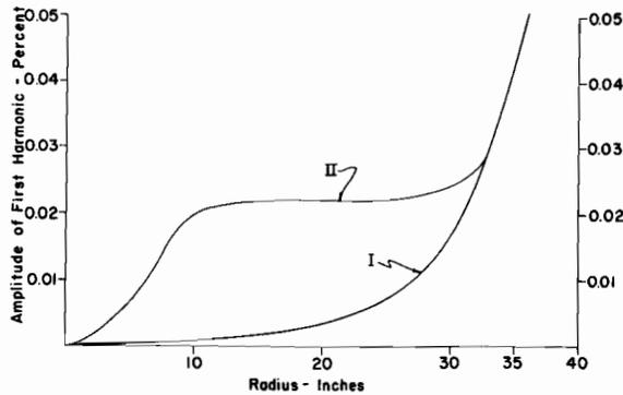
Fig. 200. Amplitude of first harmonic in magnet field vs radius. I and II are extremes which indicate the maximum estimated errors in determining the first harmonic at small radii.
