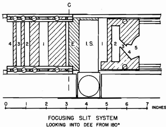
Fig. 186. Focusing grids on dee and dummy dee.
