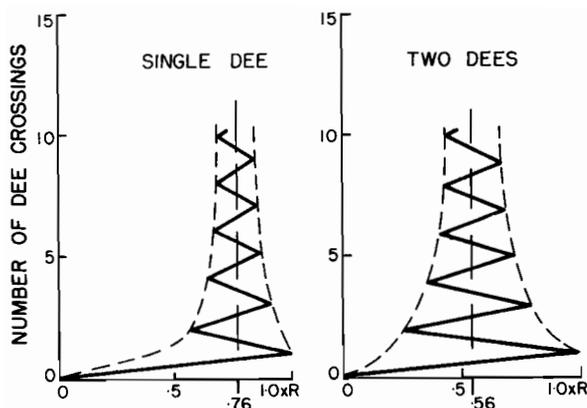
Fig. 183. Movement of orbit centers during initial motion.
