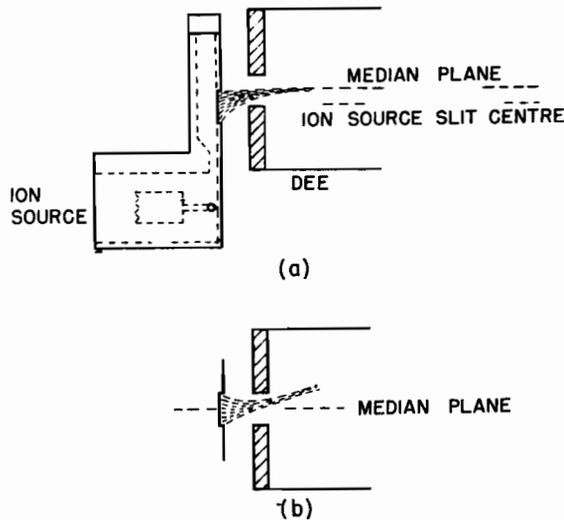
Fig. 185. Initial vertical movement of ion beam.
