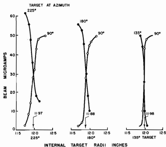
Fig. 178. Determination of three points on proton orbit.
