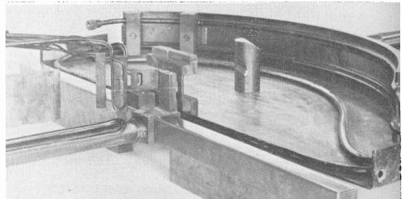
Fig. 176. Beam defining slits on first three turns.
