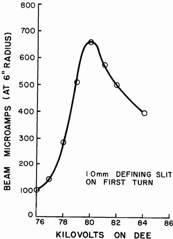
Fig. 182. Internal beam as function of dee voltage.
