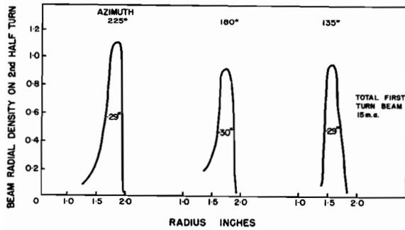
Fig. 175. Measured radial beam distribution on first turn.
