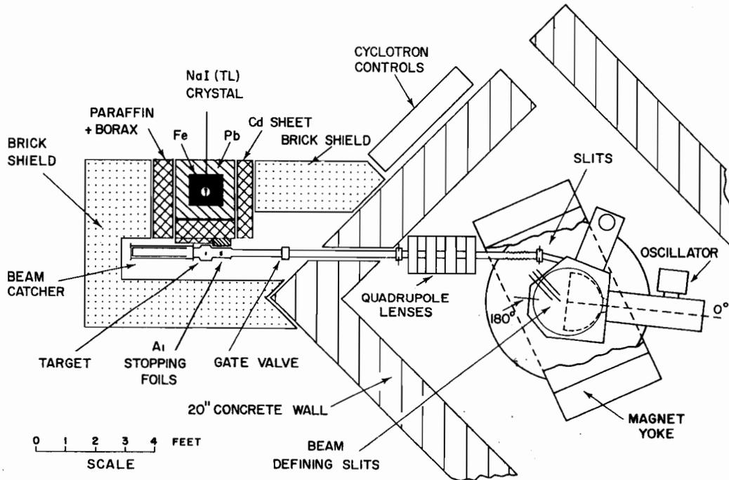
Fig. 188. Experimental arrangement for proton-capture gamma ray studies.
