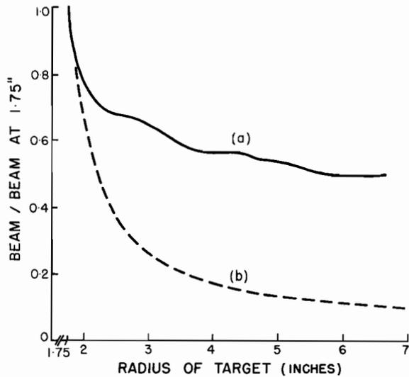
Fig. 187. Beam loss with radius, (a) with and (b) without focusing grids.
