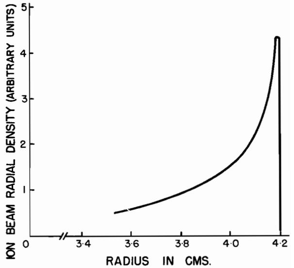
Fig. 174. Calculated radial beam distribution on first turn.
