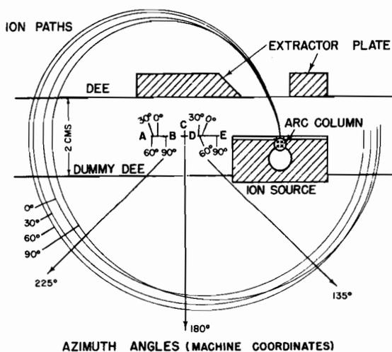
**Fig. 172. Calculated orbits near ion source.**
