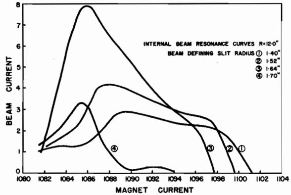
Fig. 181. Measured resonance curves.
