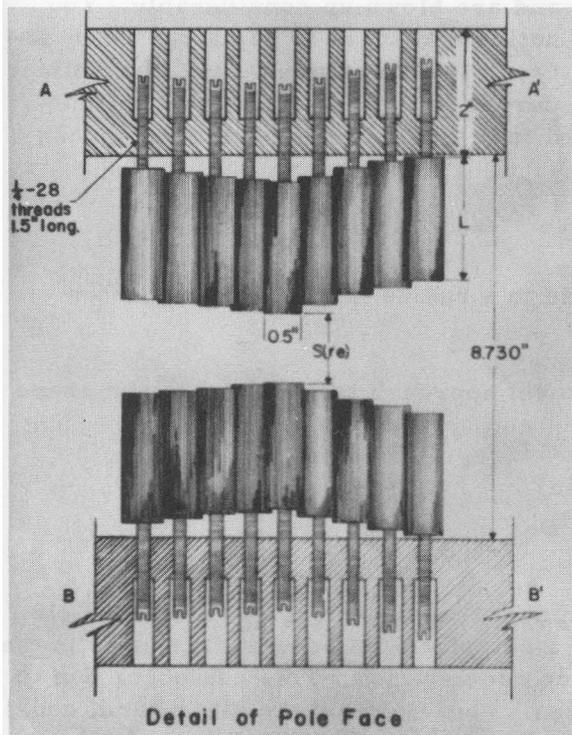
Fig. 128. Details of pole construction.
