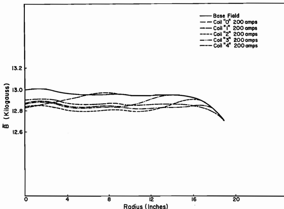
Fig. 74. A composite of the corrections produced by the five field coils. The current is 200 amperes or about 2000 amp-turns for each pair of coils. The corrections oppose the base field.
