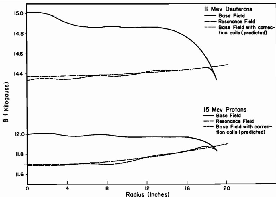
Fig. 75. Corrected field configurations for 15-Mev protons and 11-Mev deuterons.
