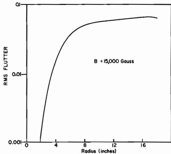
Fig. 71. A plot of the flutter against radius. The spiral shims terminate at the center in a 7-1/4-in. dia. iron disk.
