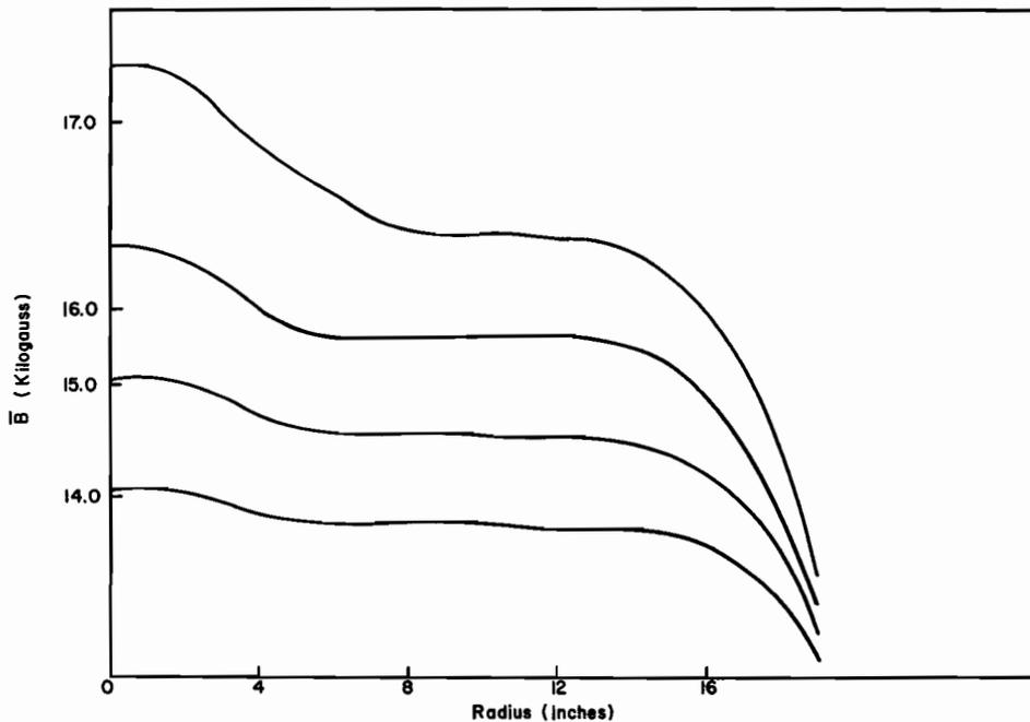
Fig. 73. The azimuthally averaged magnetic field.
