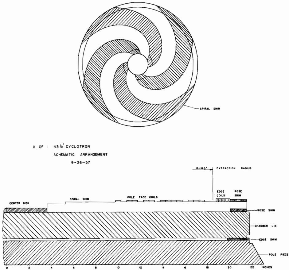
Fig. 69. The shim arrangement used in the University of Illinois 43-inch cyclotron. The shim thickness is 7/8-in. Five sets of field correction coils are required.
