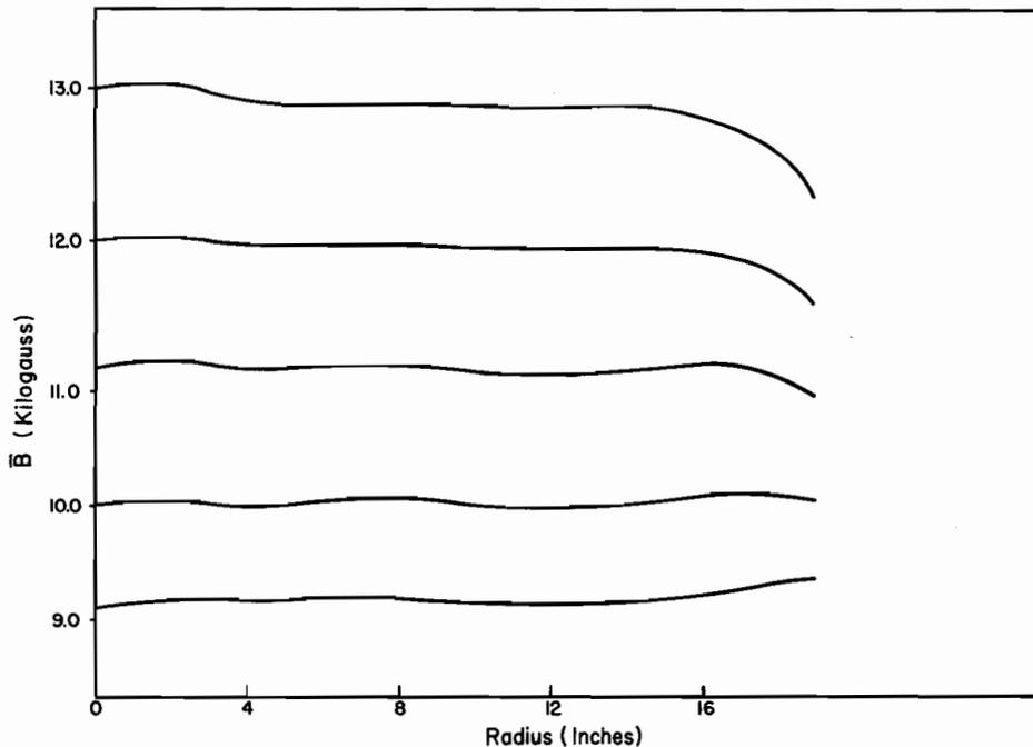
Fig. 72. The azimuthally averaged magnetic field as a function of the radius of a pole piece.
