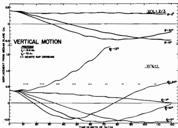
Fig. 67. Axial motion for protons. The time is in units of  $T_e/24$  where  $T_e$  is the r-f period. The upper set of curves were made for 50-kv dee voltage.
