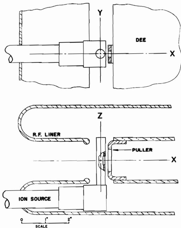
Fig. 64. Schematic arrangement of the dee liner and ion source configuration.
