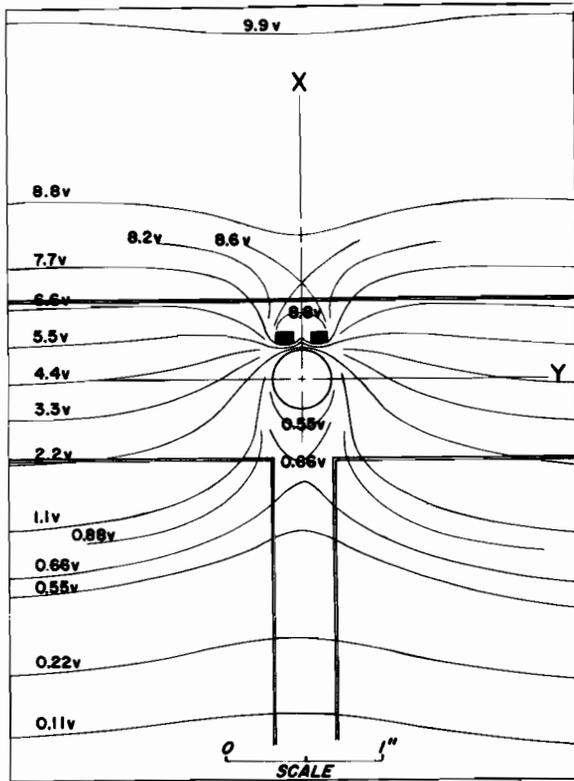
Fig. 65. Electrolytic tank measurements of the median-plane potential distribution. Dee to ground potential was set at 10 volts. Note that for all computations the ion source and puller were moved 0.5 cm toward the dummy dee to center the orbits.
