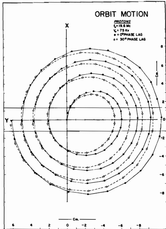
Fig. 66. Orbit motion for protons.
