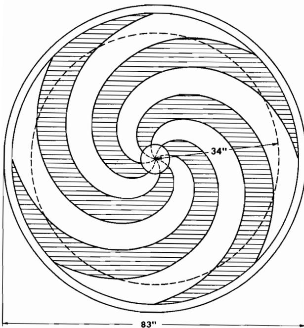
Fig. 59. Schematic diagram of a 4-spiral-sector design for 40-Mev deuterons, with flat shims cut in an Archimedean spiral.
