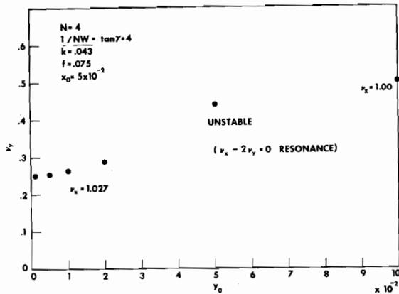
Fig. 62. y-betatron oscillation frequency as a function of initial y-amplitude.
