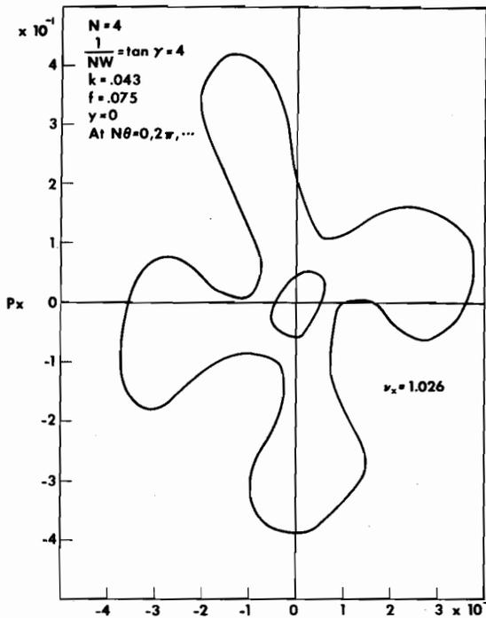
Fig. 60.  $x$ -motion phase curve;  $x$  is measured in units of the radius; the radius;  $p_x = \frac{dx}{d}$  in radians.
