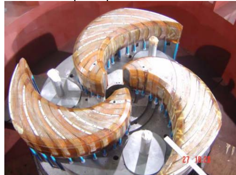
Figure 6: Trim coils placed on the pole tip.
