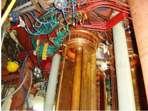
Figure 8: One of three lower outer conductor spinning assemblies below pole base of the cyclotron magnet.
