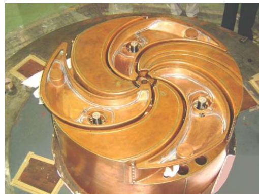
Figure 7: Liner and dees installed on lower pole tip.
