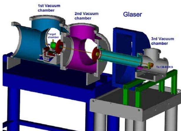
Figure 3: Light-ion guide in test set-up.
