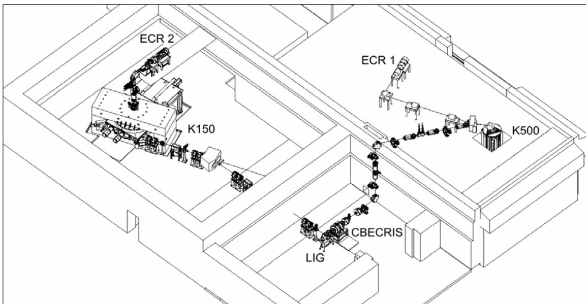
Figure 1: Layout of the scheme to accelerate radioactive beams
