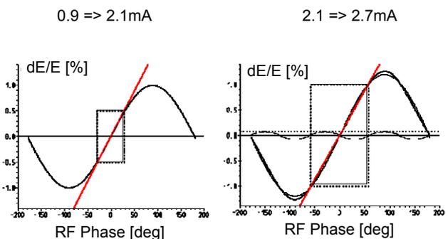
Figure 3: Widening of the linear part by applying a negative 3<sup>rd</sup> harmonic component to the buncher voltage.
