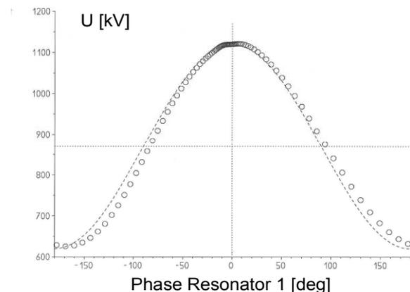
Figure 6: Energy distribution of the beam after having crossed resonator 1. The bunch is located symmetrically to the crest of the RF voltage
