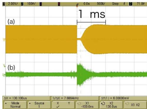
Figure 4: Instant recovery of gap voltage. a):signal from a resonator pickup loop. b):reflection signal of a directional coupler attached to the transmission line.
