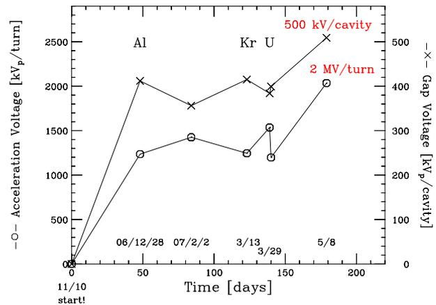
Figure 5: Improvement of the acceleration voltage.
