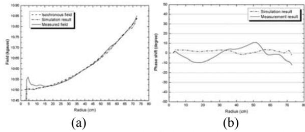
Figure 3: Average magnetic field distribution graph (a) and accumulated phase error (b).
