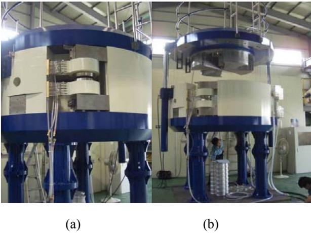
Figure 5: Photograph of operation after assembly (a) and opening upper yoke with oil pressure cylinder (b).
