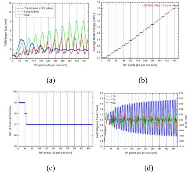
Figure 8: Change of beam size (a), energy increment of per turns (b), particle loss (c) and magnetic field (d).
