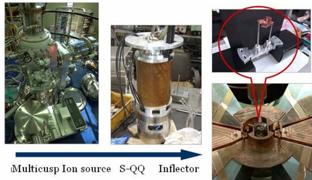
Figure 12: Manufactured photograph of Ion source, S-QQ, and spiral inflector.
