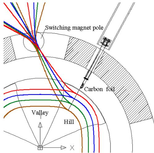
Figure 16 : Extraction position of 15 – 30 MeV.
