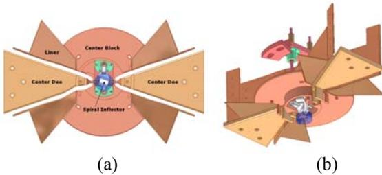
Figure 6: Central region of KIRAMS-30 (a) 3-D view of central region and spiral inflector (b).
