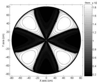
Figure 2: Magnetic field characteristics of KIRAMS-30.
