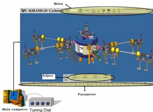
Figure 19: User interface for control program.
