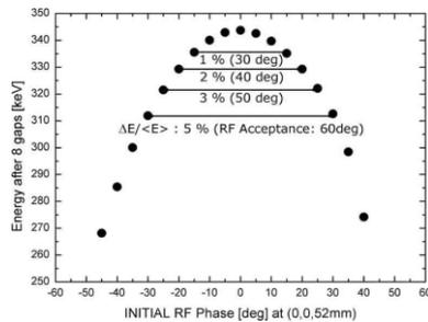
Figure 7: The results of beam train simulation and RF acceptance with several energy spreads.
