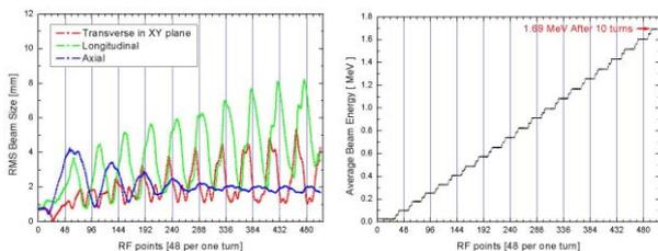
Figure 9: Beam envelope and Beam energy during 10 turns
