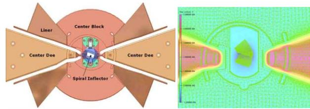
Figure 5: Drawing and E-field Distribution of the Central Region
