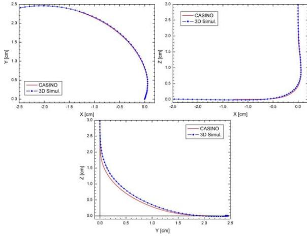
Figure 3: The Central Rays of the Spiral Inflector
