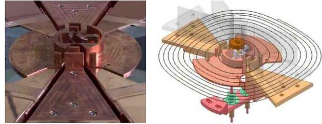
Figure 1: The Central Region of KIRAMS-30 Cyclotron
