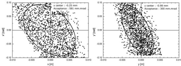
Figure 4: Beam acceptance of the spiral inflector
