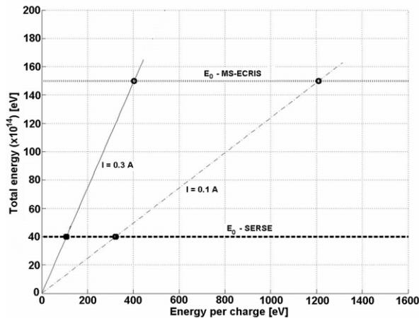
Figure 3: Comparison of total LIS beam energy and plasma energy content.
