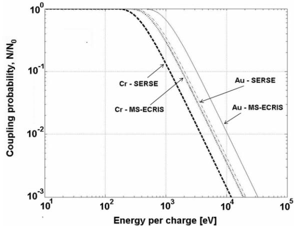
Figure 2: Coupling probability for O plasma with Cr and Au as injected ions, vs. the energy per charge.
