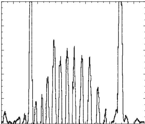
Figure 1: Typical charge state distribution for Au.
