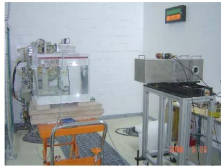
Figure 7: A setup to measure the prompt gamma distributions. Water phantom and the collimator system are shown. The CsI detector is taken out to count background radiation.
