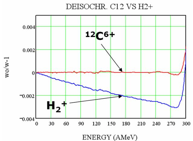
Fig. 5: The plot shows the isochronism as a function of the energy of both beams without tuning of the magnetic field. To accelerate the H<sub>2</sub><sup>+</sup> in the proper way, it requires that isochronism value ( $\omega_0/\omega - 1$ ) be less than 0.0005 as the red line shows for the carbon ions.
