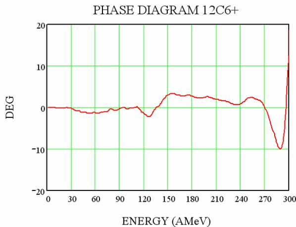
Fig.3: Phase history of carbon ion as a function of the energy. Due to the 4<sup>th</sup> harmonic operation of RF system, the phase excursion of the beam has to be kept within few degrees to get an acceptable acceleration.
