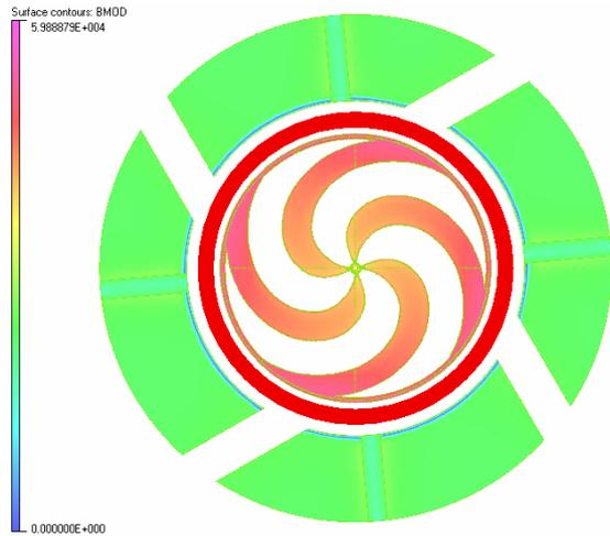
Fig.2: Top view of the magnetic field in the hills and the yoke.
