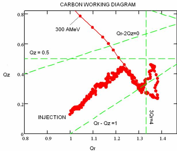
Fig.4: Working diagram of the cyclotron. The main dangerous resonance are shown as dashed green line.
