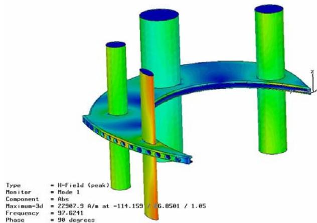
Fig.6: Current distribution on the complex DEE-stems of one cavity. As shown, four stems are expected to get the resonant frequency of 97 MHz. Due to the high value of voltage (120 KV) at the extraction region, the power dissipation on the outer stem becomes higher.
