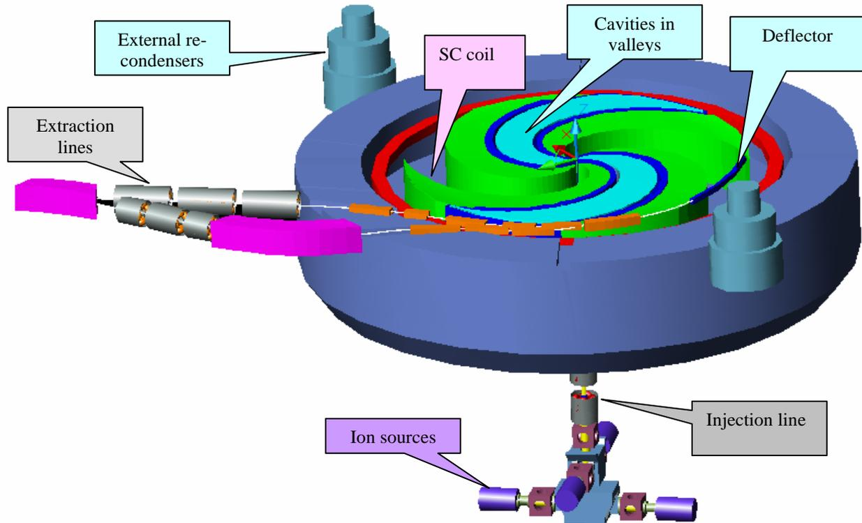
Figure 1: Artist's view of the median plane in the 400 MeV/amu Carbon/Proton superconducting cyclotron.
