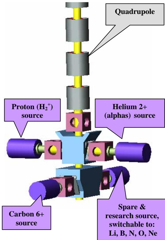
Figure 2: Injection line and ion sources.
