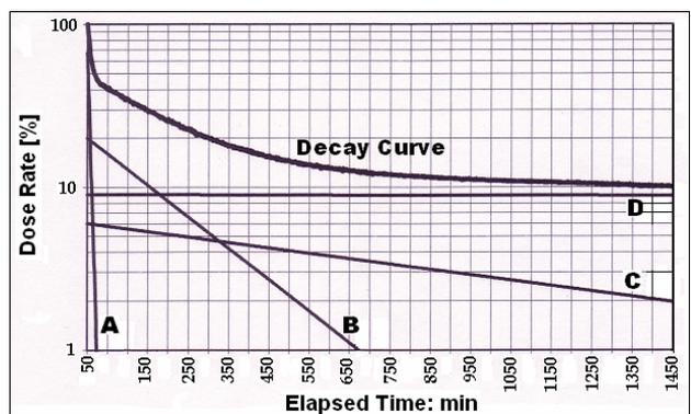
Figure 3: Normalised (%) gamma dose equivalent rate recorded with gamma area monitors is plotted as a function of elapsed time (decay curve). The decay curve was unfolded with four exponential functions (A), (B), (C) and (D), representing four major activation products.
