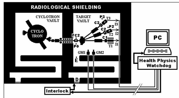
Figure 1: Footprint of the NMC Facility showing the high current SPECT (T1, T2, T3 radioisotope production target stations, collimators (C1, C2, C3) and Faraday Cup (FC2).
