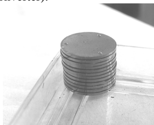
Figure 9: View of a piece of the target with 0.3 mm bumps. The target consists of 123 pellets (15 mm diam.) Each pellet is about 1 mm thick overall (0.7 mm + 0.3 mm).
