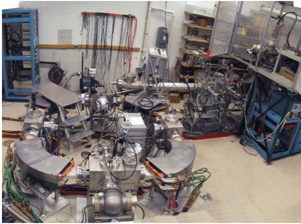
Figure 6: Photograph of the Small Isochronous Ring. The ion source is in the high voltage cage on the upper right. The extraction chamber is in the foreground. The circumference is 6.58 m.
