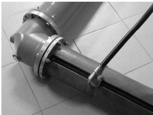
Figure 3: Photo of the detail of the connection of the dummy load cable to the slotted line.
