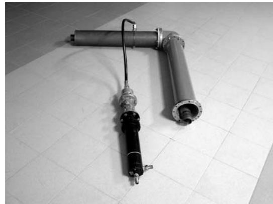
Figure 2: A photo of the 40 kW dummy load coupled to the slotted line, as a test setup arrangement for the power test of the power and driver amplifiers.
