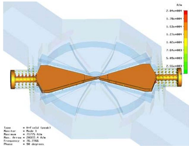
Figure 4: Magnetic field distribution
