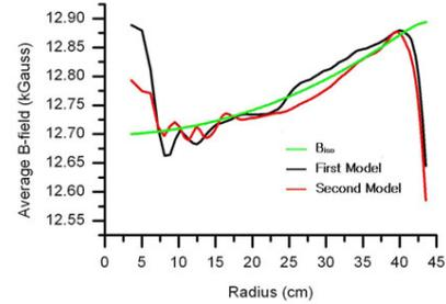
Figure 1: Average magnetic field along the average radius of the beam.
