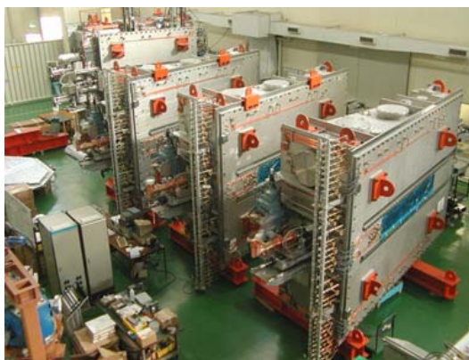
Figure 5: The rf-resonators(acceleration type I,II, and flat-top) during fabrication at Niihama works, SHI.
