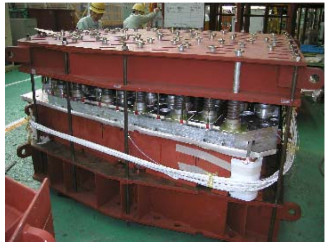
Fig. 7: A jig for cures of the superconducting trim coils.
