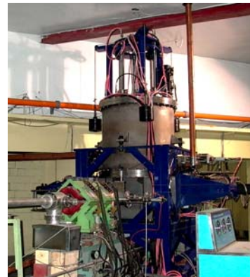
Figure3: A new rebuncher between SFC and SSC
