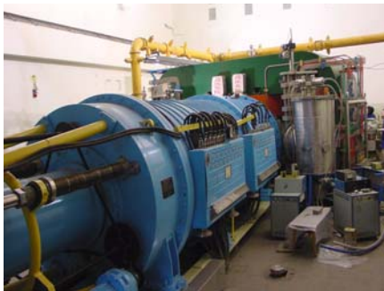
Figure2: SFC with a new vacuum chamber
