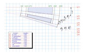
Figure 5: Plane view of the main magnet of the booster ring. Each magnet has DFD structure and the line p1in the figure is the center of the magnet, thus plane symmetry to this line.
