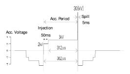
Figure 4: Acceleration pattern of FFAG injector.
