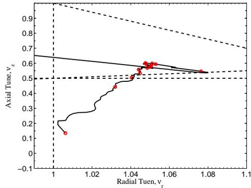
Figure 6: The operating points diagram during the acceleration and the dangerous resonances.
