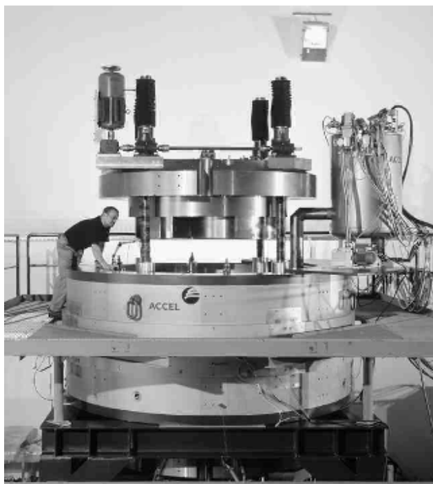
Figure 3: The 250 MeV medical cyclotron at ACCEL during cryogenic and magnetic tests.
