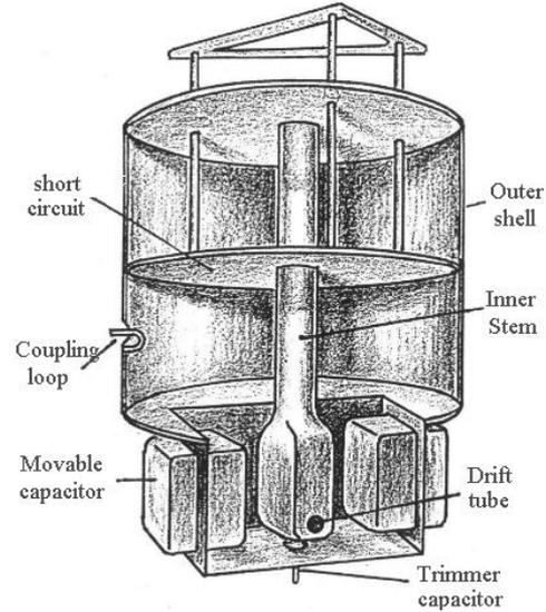
Figure 2 Schema for the B1 cavity
