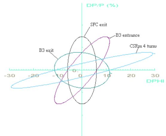
Figure 4 Phase ellipses with SFC-SSC-CSRm matching
