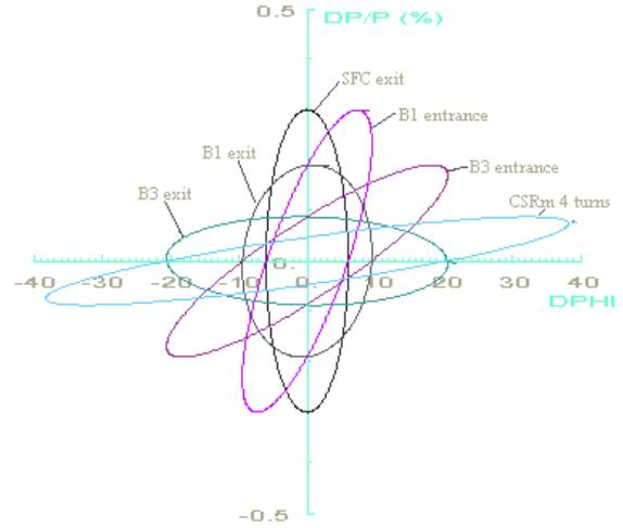
Figure 3 Phase ellipses with SFC-CSRm matching
