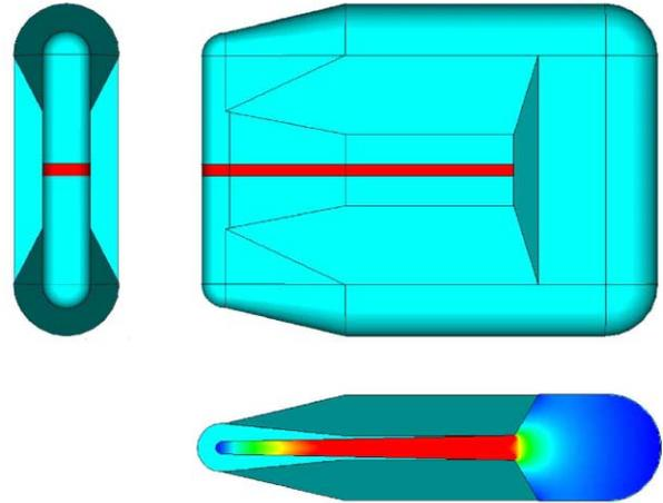
Figure 3: Proposed 50 MHz cavity for the Injector 2. Above: side and front view of the cavity. Below: the accelerating field distribution in the beam plane.
