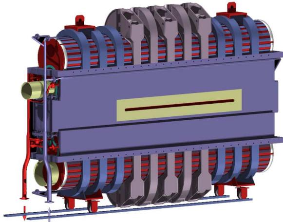
Figure 5: 50 MHz prototype cavity. The RF wall is made of 8 mm copper sheets. The support structure consists of stainless steel. The cavity can dissipate 500 kW of RF power and has a calculated shunt impedance of 1.8 M $\Omega$ .
