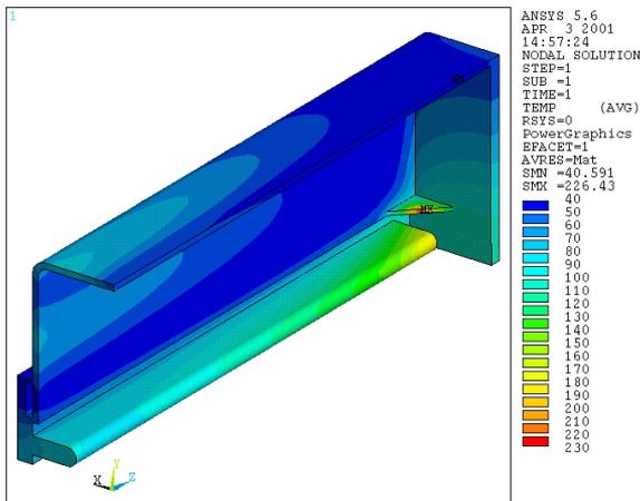
Figure 6: FEM analysis of the flattop cavity. The temperature distribution corresponds to a gap voltage of 550 kV<sub>p</sub> (Dissipated RF power of 95 kW).
