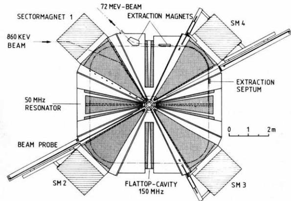
Figure 2: Layout of the Injector Cyclotron (72 MeV<sub>p</sub>)
