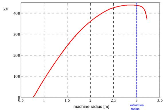
Figure 4: Radial Distribution of the Gap Voltage. The values correspond to a dissipated RF power of 100 kW in the cavity.
