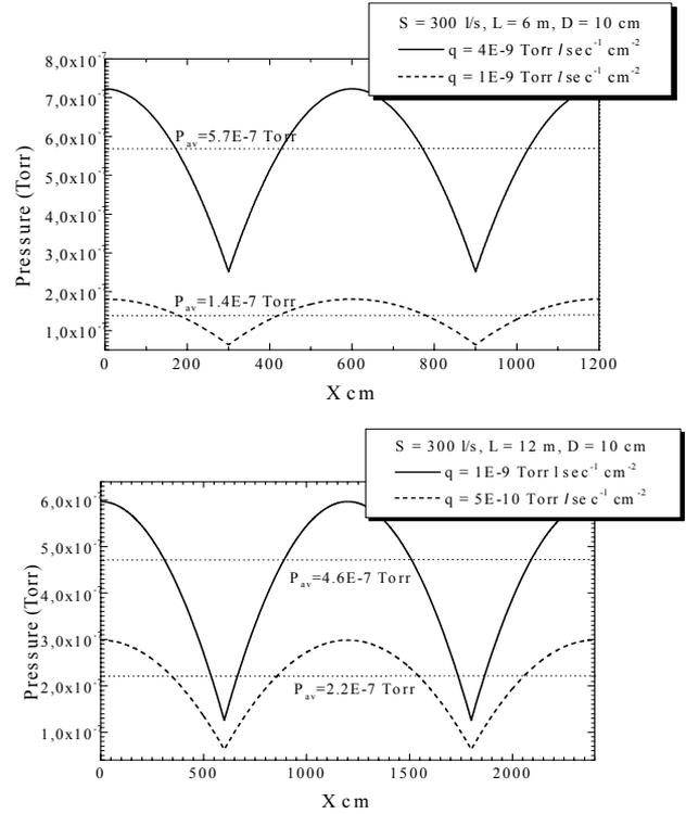
Figure 3: Pressure distribution for the periodic distances of 6 m and 12 m between the pumps (each of 300 l/s effective pumping speed) and its dependence on the specific outgassing.
