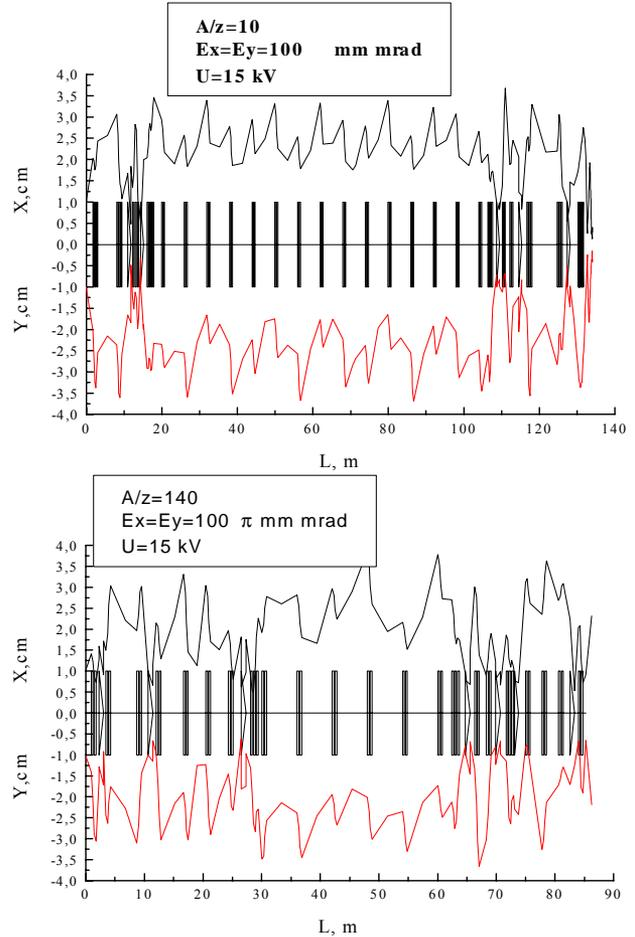
Figure 4: Beam envelopes along the transport lines of Phases 1 and 2.
