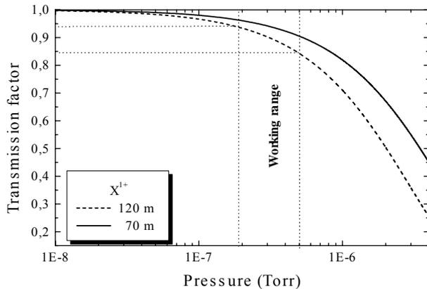
Figure 2: Transmission factor versus average pressure for beam lines of 70 m and 120 m in length.
