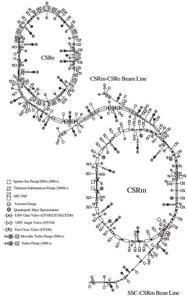
Figure 1: The vacuum equipment layout of HIRFL-CSR
