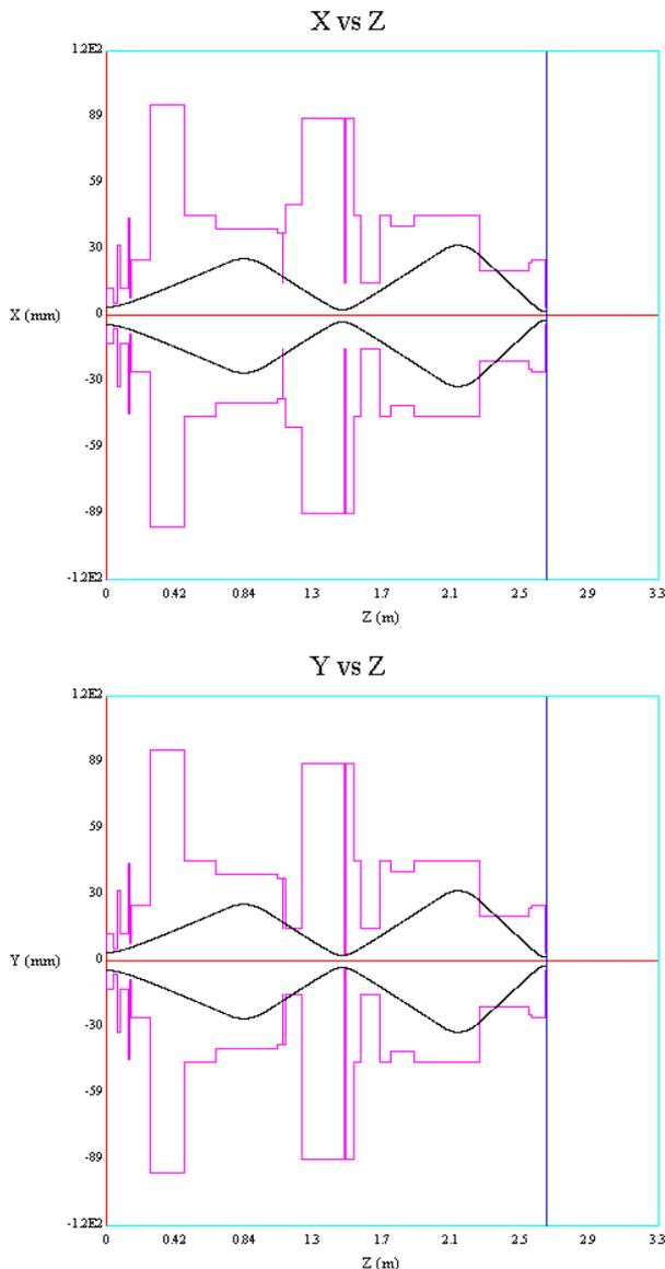
Figure 3. Horizontal and Vertical Beam Profiles in the TR9DP Injection System.
