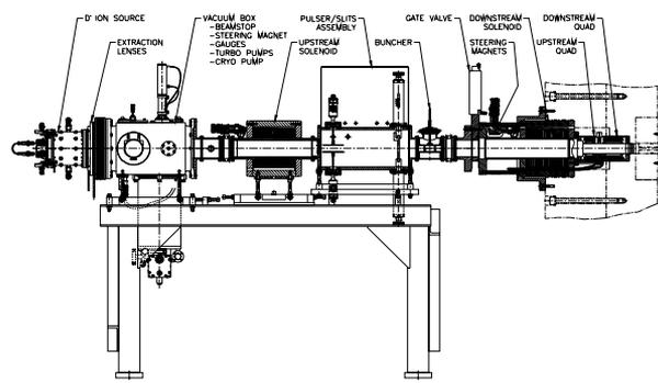
Figure 2. Layout of TR9DP Ion Source and Injection System.
