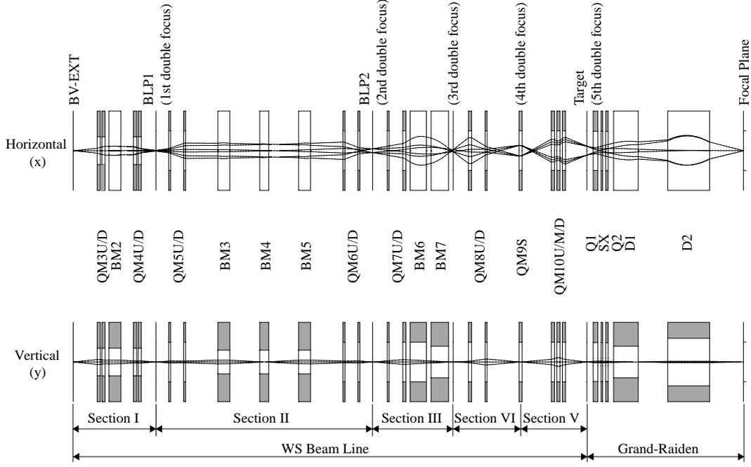
Figure 1: Envelopes of dispersive beam in the horizontal and vertical planes from the object point at the exit of the Ring Cyclotron (BV-EXT) via the target location to the focal plane of the Grand Raiden spectrometer. Trajectories are shown for particles with  $\Delta p/p = \pm 0.03\%$ ,  $\Delta\theta = \pm 2$  mrad, and  $\Delta\phi = \pm 2$  mrad. The transverse scale is increased for illustration purposes.
