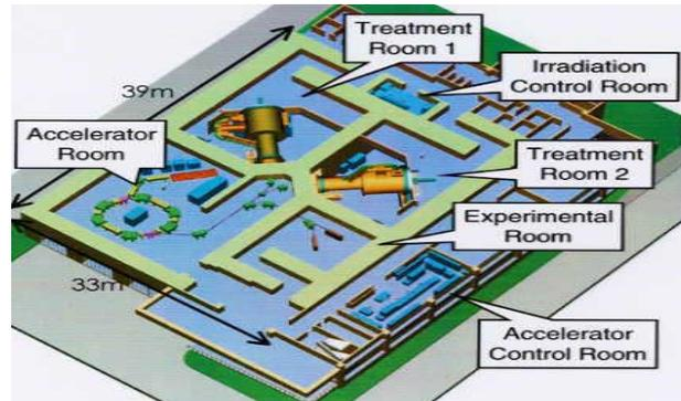
Fig. 12: Bird's Eye View of Tsukuba Proton Therapy facility.
