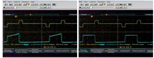
Figure 6: (Color) A proton beam with profiles before (left) and after (right) profile-unevenness compensation.
