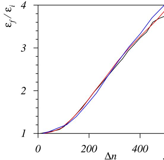
Figure 5: Final rms emittance growth factors as function of  $\Delta n$  and for different space charge tune shifts (0.2/black, 0.4/red, and 0.8/blue)
