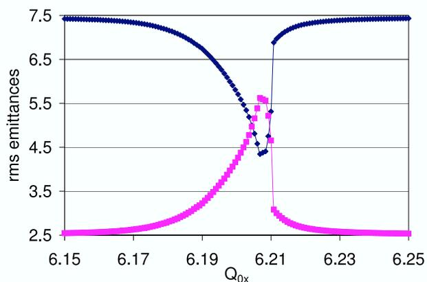
Figure 1: Static tunes stop-band: final rms emittances for different values of  $Q_{0,x}$ .
