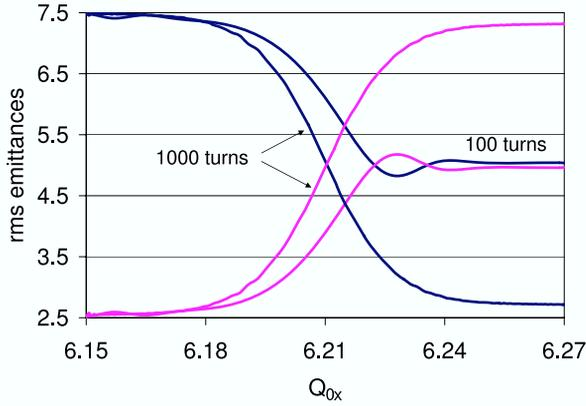
Figure 2: Evolution of emittances by crossing the stop-band dynamically from below over 100 and 1000 turns.
