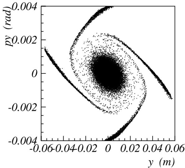
Figure 4: Vertical phase space plot after crossing the resonance condition  $Q_{0,y} = 3$ .
