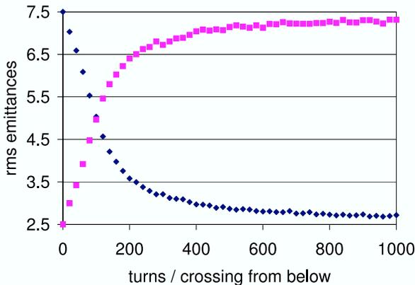
Figure 3: Final emittances after crossing  $Q_{0,x} = 6.15 \rightarrow 6.27$  at variable rates.
