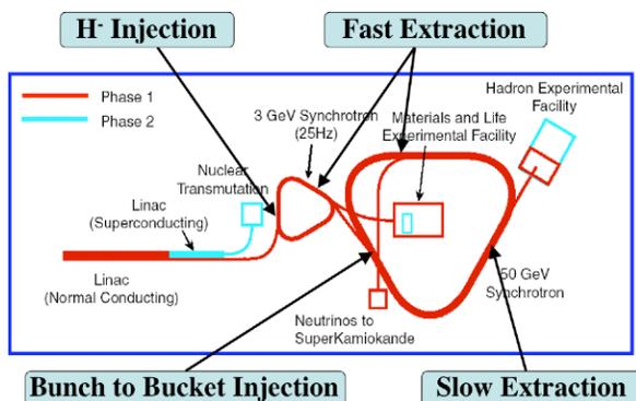
Figure 1: Layout of the J-PARC accelerator complex and locations of injections and extractions.
