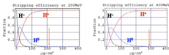
Figure 4: Charge state fraction as a function of the thickness of the carbon foil for 200 and 400 MeV energy.
