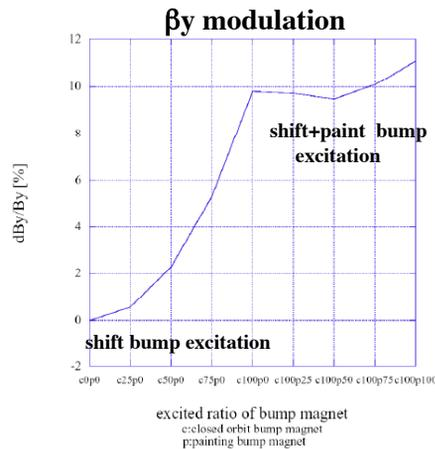
Figure 6:  $\beta_y$  modulation produced by the shift/paint bump magnets during injection time.
