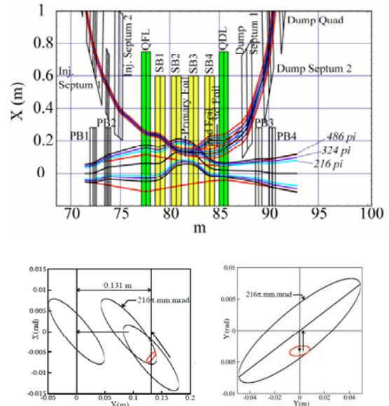
Figure 2: Injection layout of the J-PARC RCS [2] and phase space relation between linac beam and painted beam [3].
