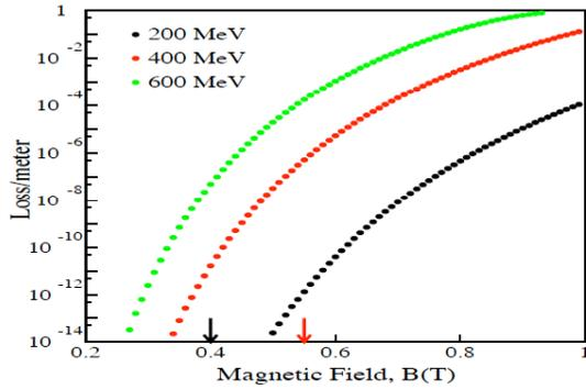
Figure 3: Fractional beam loss per meter by Lorentz stripping as a function of the magnetic field.
