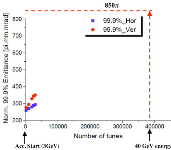
Figure 9: Long term space charge simulation during acceleration for the J-PARC main ring.
