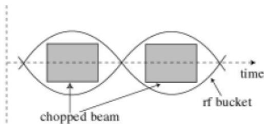
Figure 7: Chopped beam and rf bucket.
