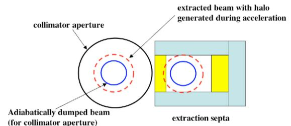
Figure 8: Relation between the beam size, the collimator and the extraction aperture.
