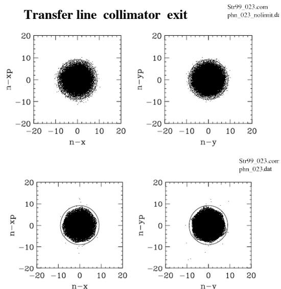
Figure 10: Simulation of the beam halo scraped by the collimators located the transfer line from the J-PARC RCS to MR.
