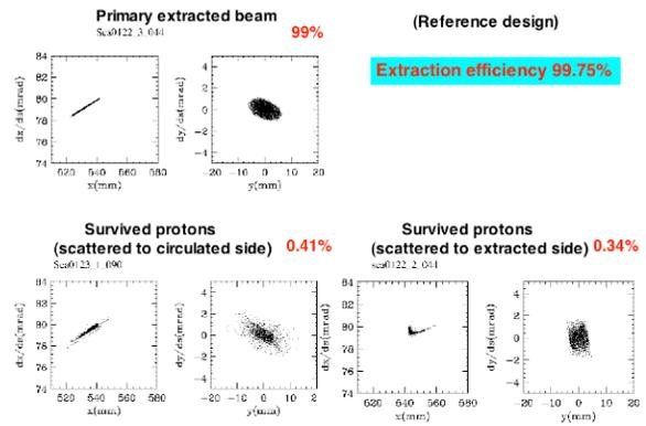
Figure 12: Phase space distributions of primary and halo beam extracted from the J-PARC. The beam halo is generated by the scattering on the ESS wires.
