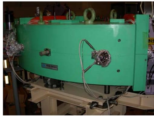
Fig. 5 Vacuum window to guide the laser inside of the S-LSR vacuum system. The window is to be replaced by the one suited for laser guiding at the next vacuum breaking.
