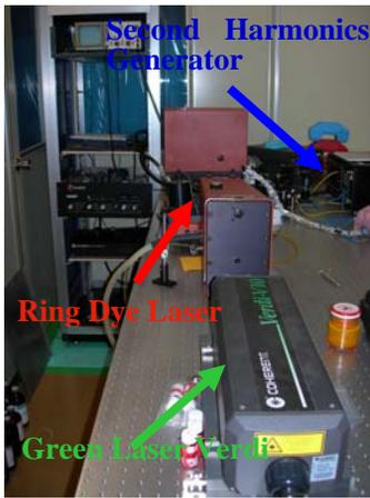
Fig.4 Ring dye laser tuned up for laser cooling.
