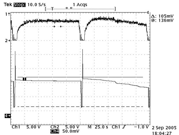
Figure 4: Electron cooling at 70 keV again with 250 mA electron current but in the first cycle with a slightly 0.35 mrad horizontally misaligned electron beam. No coherent oscillations at all. In the following cycle the misalignment was removed resulting again in coherent oscillations as observed by the betatron frequencies seen in the transverse Schottky signal.
