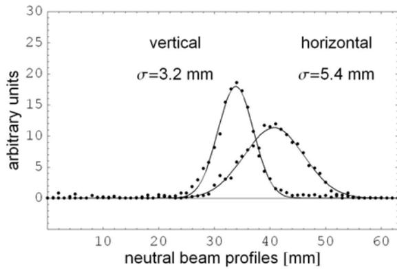
Figure 5: Horizontal and vertical  $H^0$  profiles with a 0.35 mrad horizontally misaligned electron beam. Electron beam current 130 mA. Here, the  $2\sigma$  emittances are  $\epsilon_x = 1.6 \mu\text{m}$  and  $\epsilon_y = 0.8 \mu\text{m}$ .
