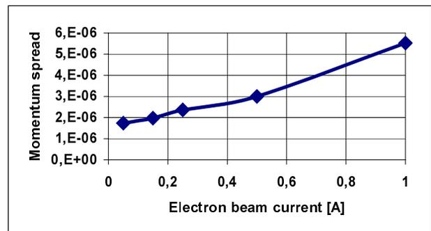
Figure 9: Dependence of minimum momentum spread on electron beam current.
