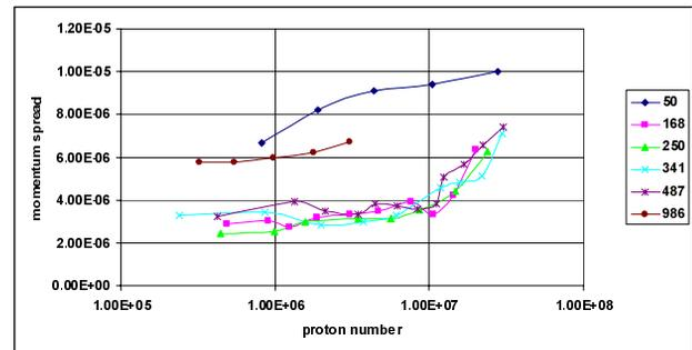
Figure 8: Cooling run 2006: Dependence of momentum spread on proton number for different electron beam current (higher vacuum pressure of  $10^{-7}$  mbar in the target telescope section due to an air leak).
