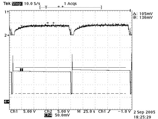
Figure 3: Electron cooling at 70 keV electron energy with 130 mA electron current. No coherent oscillations at all. The slight, exponential decrease of the proton intensity within the 2 min cycle is interpreted as single scattering beam loss due to the residual gas in the 183 m long COSY ring, which had a mean pressure of about  $2 \times 10^{-9}$  mbar.
