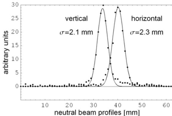
Figure 2:  $H^0$  beam profiles corresponding to the well cooled beam in Fig. 1 measured at about 30 s after injection before onset of the horizontal oscillation. Lattice model based optical functions at the position of the electron cooler ( $\beta_x = 9$  m,  $\beta_y = 18$  m,  $D = -6$  m) yield  $2\sigma$  emittances of  $\epsilon_x = 0.28 \mu\text{m}$  and  $\epsilon_y = 0.35 \mu\text{m}$ .
