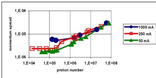
Figure 7: Cooling run 2005: Dependence of momentum spread on the proton number for different values of electron beam current (vacuum pressure  $10^{-9}$  mbar).
