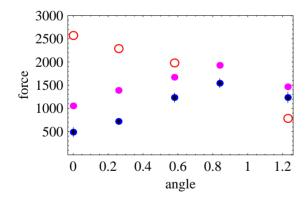
Figure 5: Longitudinal force [eV/m] vs angle [rad] for ion velocity of  $V = 3 \cdot 10^5$  m/s, and zero-temperature electrons. VORPAL results: dots with error bars - B=5T, dots without error bars - B=1T, open circles - B=0.1T.
