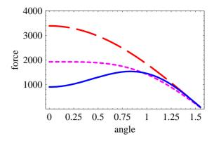
Figure 6: Longitudinal force [eV/m] vs angle [rad] for ion velocity of  $V = 3 \cdot 10^5$  m/s, and zero-temperature electrons. Derbenev-Skrinsky-Meshkov asymptotics [9] results: blue (solid) line - B=5T, pink (dash) curve - B=1T, red (dash dot) curve - B=0.1T.
