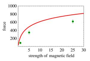
Figure 7: Longitudinal friction force [eV/m] for  $(V_{ion,\parallel}, V_{ion,\perp}) = (3 \cdot 10^5, 0)$  m/s vs magnetic field B [T], for the finite temperature electron beam with  $(\Delta_{e,\parallel}, \Delta_{e,\perp})=(1 \cdot 10^5, 1 \cdot 10^7)$  m/s. Solid curve - Eq. (4); dots with error bars - VORPAL results.
