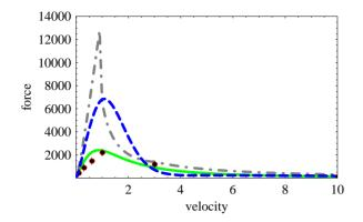
Figure 1: Longitudinal component of the force [eV/m] vs velocity  $[\times 10^5 \text{ m/s}]$ . Asymptotic expressions [9] - dotdash line (gray); Eq. (1) without the non-logarithmic term - dash line (blue); Eq. (4) - solid line (green); VORPAL results - dots with error bars.
