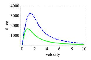
Figure 3: Longitudinal component of the force [eV/m] vs velocity  $[\times 10^5 \text{ m/s}]$  for  $\theta = 45$  degrees. Eq. (1) without the non-logarithmic term - dash line (blue); Eq. (4) - solid line (green).
