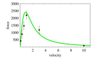
Figure 2: Longitudinal component of the force [eV/m] vs velocity  $[\times 10^5 \text{ m/s}]$  for zero transverse angle  $\theta = 0$  with respect to the magnetic field lines. VORPAL results: dots with error bars; Eq. (4) - solid line.
