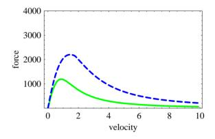
Figure 4: Longitudinal component of the force [eV/m] vs velocity  $[\times 10^5 \text{ m/s}]$  for  $\theta = 60$  degrees. Eq. (1) without the non-logarithmic term - dash line (blue); Eq. (4) - solid line (green).
