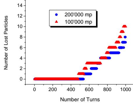
Figure 2: Particle losses for different number of macro-particles ( $10e4$  and  $20e4$ ), represented the beam.
