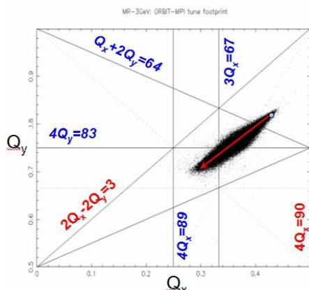
**Figure 1:** Space charge detuning for the 1.8kW/bunch beam power at the energy of 3GeV ( $B_f=0.2$ , the matched distribution in the longitudinal phase plane), including the beam environment with the rectangular chamber shape.
