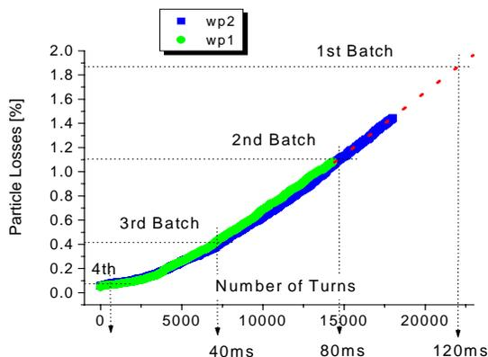
Figure 5: Particle losses for full injection time for different ‘bare’ working for the ring with the injection ‘dogleg’ including measured sextupole field component of the bending magnets and errors of the sextupole strength. Duration of the injection process for different batches of the beam is shown.
