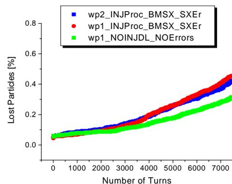
Figure 4: Particle losses at the MR scraper with acceptance of  $70 \pi$  mm.mrad for different cases.
