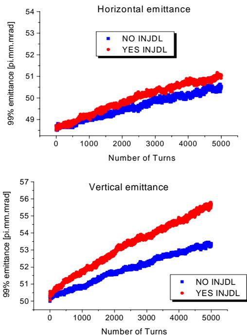
Figure 3: Emittance growth at the beginning of the injection process without and with Injection dogleg.
