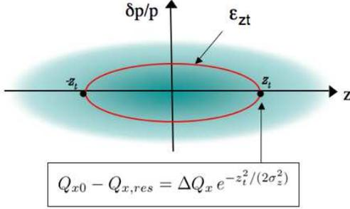
Figure 3: Schematic of the transition emittance  $\epsilon_{z_t}$  and relation between  $z_t$  and  $\epsilon_{z_t}$ .
